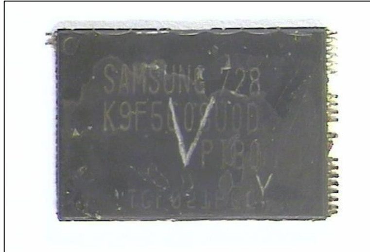
Image No. K8: Helicopter registration B516 missing pins from MPFR non-volatile memory device due to corrosion
