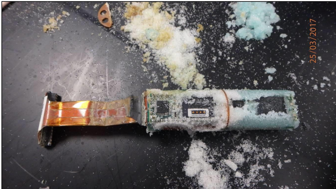
Image No. K7: APMB from EI-ICR showing copper based insulation staining of glass beads
